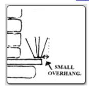
Stick the base of the bird spike level with the edge of the pipe or ledge, so that there's a slight overhang of the spike pins. Press the base down firmly so that the glue oozes out through the little holes.
