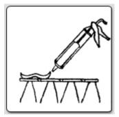
Squeeze the bird spike fixing silicone generously onto the base of the spike (thicker if the surface of the ledge is uneven).
