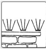
For very wide ledges, 3 or more rows of bird spikes will be necessary. Note: make sure the gap between rows is no greater than  $2\frac{1}{2}$  inches or 4-5 cm.
