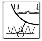
Grooves along the base of the bird spike enable them to snap into segments to fit small gaps.
