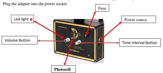
2. Led light • indicator located in front of the device flashes at a speed based on the Time Interval. The longer the interval time, the slower the flashing will be. The Time Interval can be set from 5 to 30 minutes by adjusting the knob clockwise. Similarly, you may also adjust the volume control.
